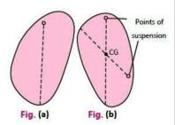
through different points (Fig. a). Each time the object is suspended, its centre of gravity lies on the vertical line drawn from the point of suspension using a plumbline. (i)
