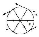
shown in figure the direction of the tangent at each point on the circle is different, the velocity is constantly changing. Hence, a force perpendicular to the direction of motion is always required to keep the object moving with uniform speed in a circular path.
