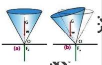
along the same vertical line. However, even a slight tilt causes it to fall over, because its centre of mass no longer remains above the base.
