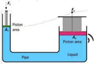
Consider a specially designed Container with two cylinders connected by a pipe as shown in figure. The smaller cylinder has a cross-sectional area  ${\cal A}_1$  and the larger cylinder has a  $\mathbf{A}_2$ . Both are filled with an incompressible liquid.
