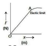
exceeds the elastic limit of the suring, it is permanently deformed and its graph will no longer remain linear. The gradient or slope of the force-extension graph is a measure of spring constant k.
