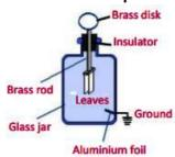
Charges can move freely from the disk to the leaves through the rod. A thin aluminium foil is attached on the lower portion of the inside of the jar. Usually, the aluminium foil is grounded by connecting a copper wire. This protects the leaves from the external electrical disturbances.
