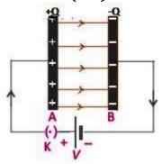
plates is air or a sheet of some insulator. This mediun is known as dielectric. It works on principal electrostatic induction.
